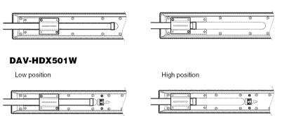
After attaching the post to the base, you can adjust the height of the speaker.
